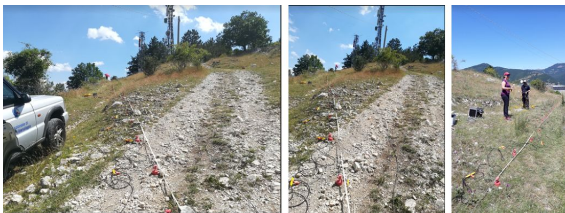
Figure 7. Photos showing the linear array of geophones (on the left and middle panel, the picture is taken in proximity of the last geophone Geo72). The Antenna area is also visible.
