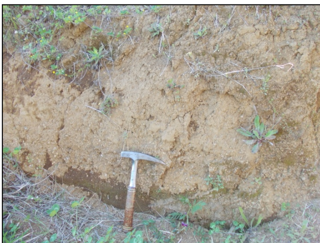
Figure 2 – Outcrop of a scarcely coherent volcanoclastic deposit close to the LAV9 station.
