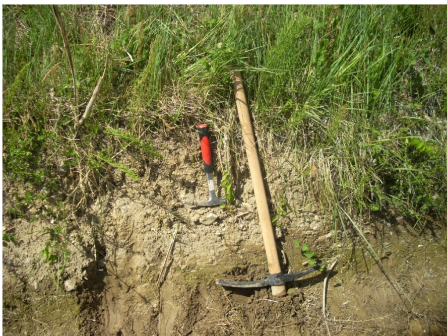
Figure 11 – 1 st order terraced alluvial gravelly-sandy deposits, gradually change to underlying silty-clayey sediments.
