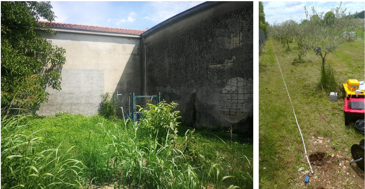
Figure 7: Left: IV.TREG accelerometric station installed in the municipality of Tregnago (VR). Right: MASW acquisition line with 2.5 m receiver spacing.
