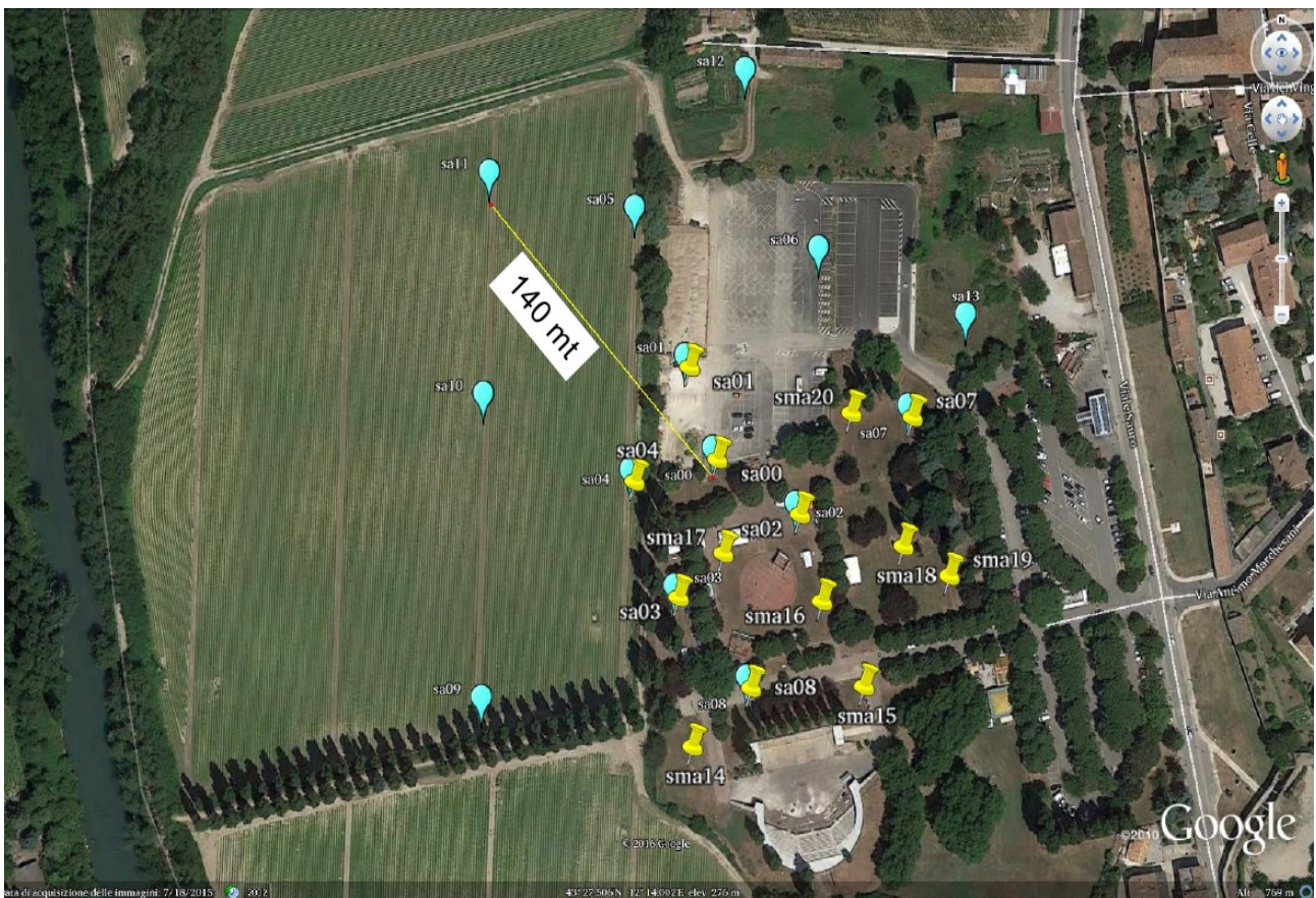
Figure 1: Plan view of the two 2D seismic arrays deployed around IV-CMPO site. The yellow and cyan points indicate the fourteen stations of the 2D array in passive configuration (named “small” and “big” array, respectively). All stations are equipped with Reftek R130 digitizer and Lennartz 3D-5sec velocimetric sensors. IV-CDCA station is situated in proximity of the sa00 station.
