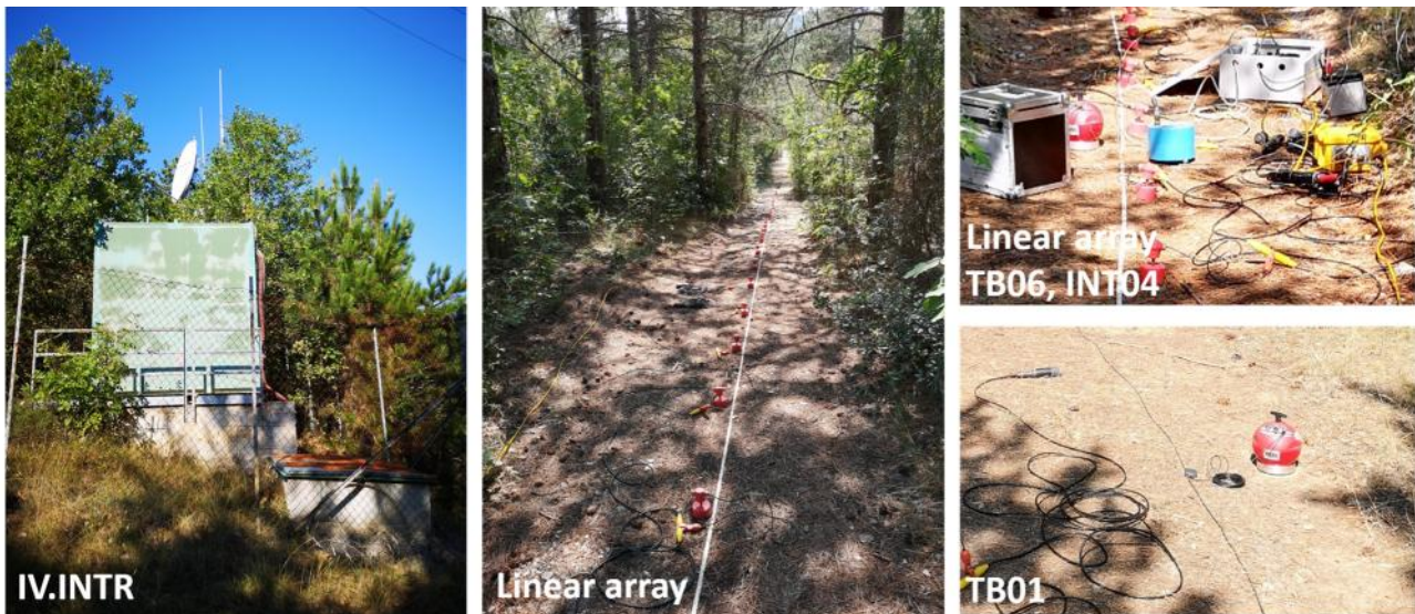
Figure 7. Pictures taken during the measurements day: (left) site hosting the IV.INTR seismic station; (middle) linear array; (right) examples of temporary seismic stations in ambient noise acquisition on 17 September 2020.
