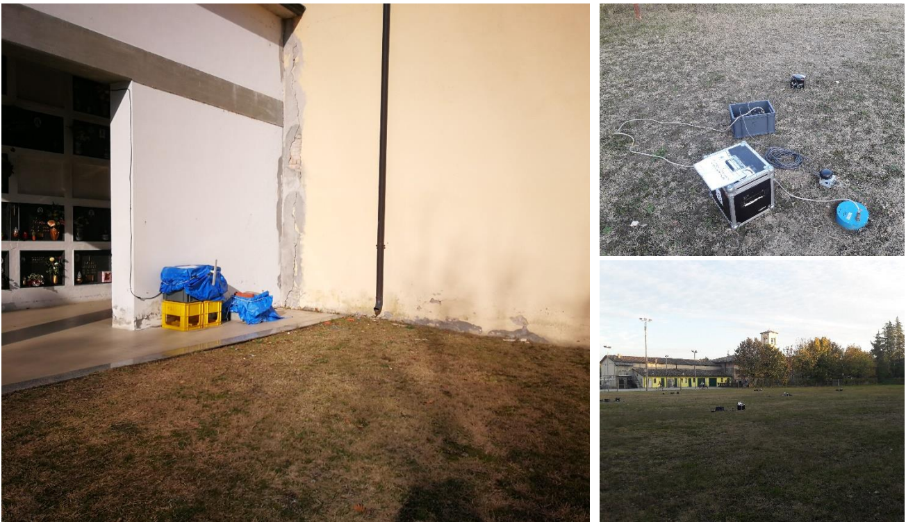
Figure 8: Left: IV.NEVI accelerometric station installed inside the municipal cemetery of Neviano degli Arduini (PR). Upper right: single station ambient noise measurement performed at IV.NEVI station. Bottom right: 2D passive ambient noise array installed close to the IV.NEVI station.
