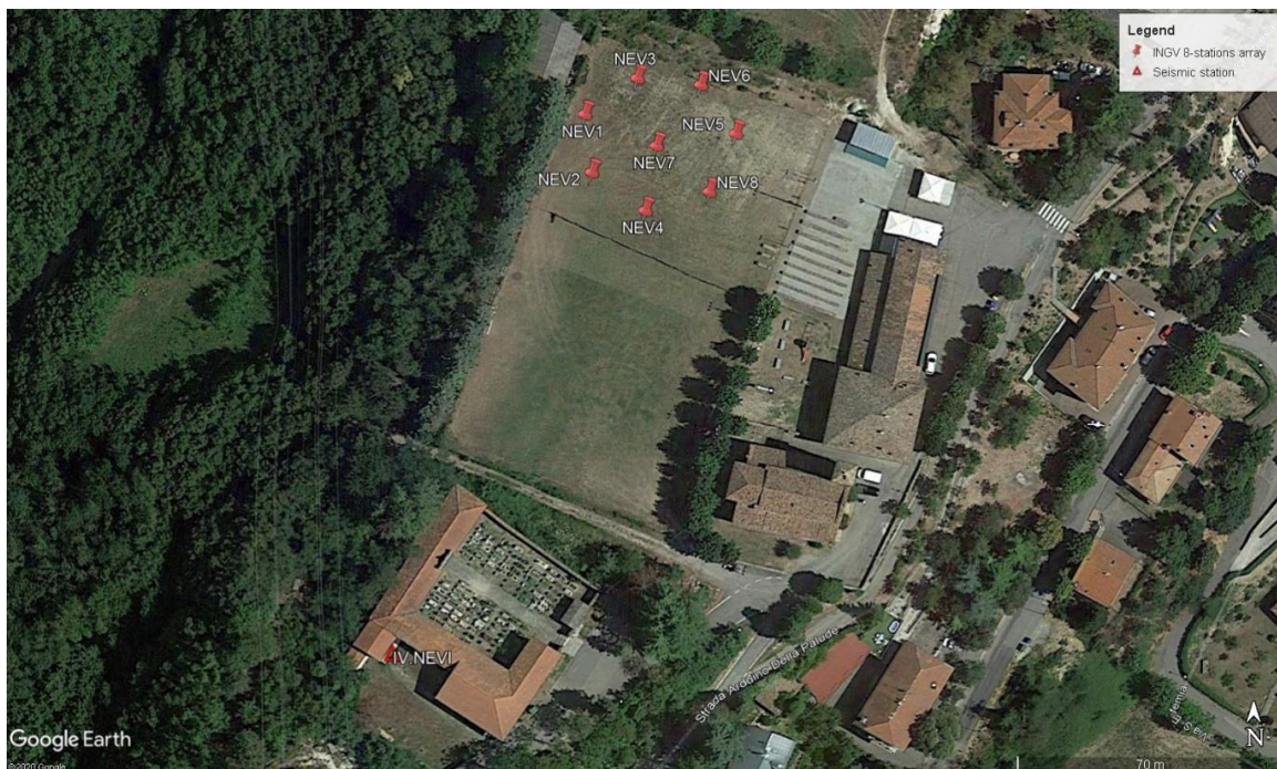
Figure 7: Map of the geophysical measurements performed at the IV.NEVI site. The red placemarkers in circular geometry are the 8 stations of the 2D array in passive configuration. The triangle indicates the IV.NEVI accelerometric station (image from Google Earth http://www.earth.google.com ).
